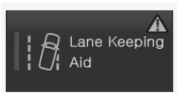
means not that the vehicle is heading out of lane but rather that the lane keeping aid is faulty.<sup>5</sup>
