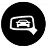
means “Side assist currently unavailable. Refer to instrument cluster display for more details.”<sup>4</sup>
